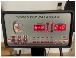
12. Pull Distance Gauge out and put to Flange – note distance on distance gauge. The number on the right must match the number noted on the distance gauge.
